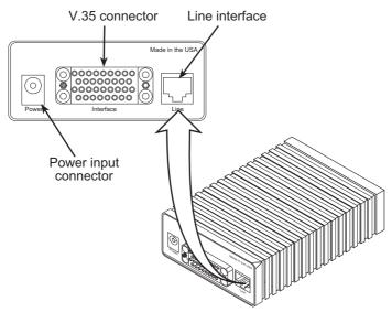
Figure 4. Model 1082 or Model 1082/144 rear view
